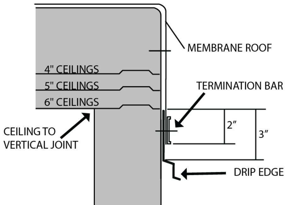
NOTE: THE DRIP EDGE SHOULD BE INSTALLED BEFORE ATTACHING THE DOWNWARD EDGE OF THE MEMBRANE ROOF. ALIGN THE TOP OF THE DRIP EDGE WITH THE CEILING TO VERTICAL JOINT. ATTACH DRIP EDGE AT TWO OR THREE LOCATIONS TO TEMPORARILY HOLD IT IN PLACE. NOW COMPLETE INSTALLATION OF MEMBRANE ROOF.
